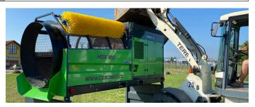
fferent sieves on the drum with different sizes of the sieve openings. This concept makes possible screening up to 4 different fractions. High efficiency of screening is secured by drum rotation speed control, conveyor speed control and possibility to change angle of the fins for pushing the material inside the drum. Cleaning of the drum is handled by built-in rotation broom.
